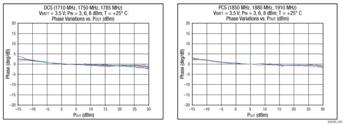
Figure 3. Typical AM/AM and AM/PM Response Charts for High Band - SKY77336 Power Amplifier Module
