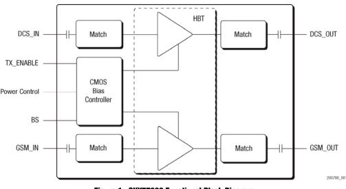
Figure 1. SKY77336 Functional Block Diagram
