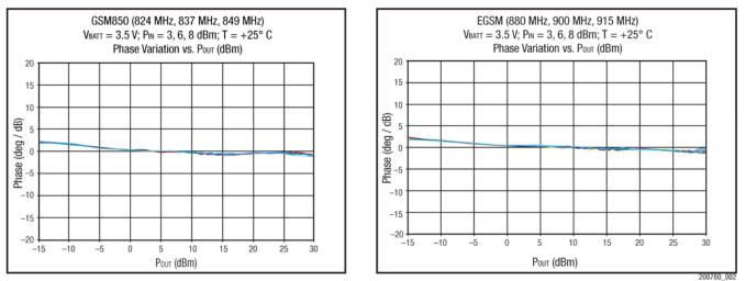
Figure 2. Typical AM/AM and AM/PM Response Charts for Low Band – SKY77336 Power Amplifier Module
